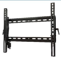
Universal tilting mount with lock for 26'' to 55'' displays. Adjustable tilt wall mount with Universal hole pattern to fit a wide selection of diplays. Smooth tilt adjustments of  $15^\circ$  forward and  $5^\circ$  back with a locking knob for a variety of viewing angles. Makes a secure installation quick and easy, simply hang the display and turn the pre-assembled securing screw to lock in place. Open wall plate design provides easy access to wiring.
