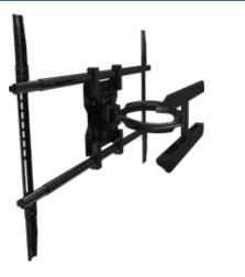
Pivoting mount for 37" to 80"+ flat panel displays\*. Swinging arm holds display 3.5" from wall and extends up to 14.5". Smooth tilt adjustments of 15° forward and 5° back with a locking knob for a variety of viewing angles. 3° side to side roll for perfect positioning. Makes a secure installation quick and easy, simply hang the display and turn the pre-assembled securing screw to lock in place. Integrated cable management for clean look.
