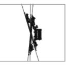
**Tilt** 15° forward and 5° back tilt for optimal viewing angles.
