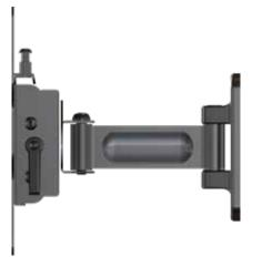
Pivoting mount for 13" to 49" flat panel displays\*. Swinging arm holds display 2.8" from wall and extends up to 7.9". Smooth tilt adjustments of 15° forward and 5° back with a locking knob for a variety of viewing angles. 5° side to side roll for perfect display positioning. Makes a secure installation quick and easy, simply hang the display and turn the pre-assembled securing screw to lock in place. Integrated cable management for clean look.
