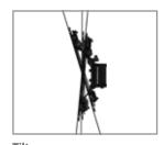
111t 15° forward and 5° back tilt for optimal viewing angles.
