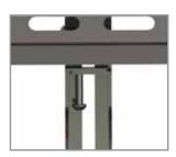
**Pre-Installed Securing Screws** *Easy hook and secure installation and pre-assembled securing screws makes installation fast and easy.*
