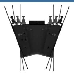
Ceiling mount box and VESA display adapter assembly for 13″ to 46″ dual back to back displays. Attaches to standard 1.5″ threaded extension columns. Continuous tilt of 20° forward with 360° rotation. Makes a secure display installation quick and easy, simply hang the display and turn the pre-assembled securing screw to lock the VESA adapter in place. Compatible with all 1.5″ NPT threaded pipe.
