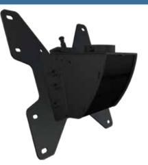
Ceiling mount box and VESA display adaptor assembly for 13" to 46" displays\*. Attaches to standard 1.5" threaded extension columns. Continuous tilt of 20° forward with 360° rotation. Makes a secure display installation quick and easy, simply hang the display and turn the pre-assembled securing screw to lock the VESA adapter in place. Compatible with all 1.5" NPT threaded pipe.
