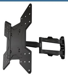
Articulating mount for 13" to 55" displays\*. Multiple joint arm holds display 2.7" from wall when retracted and 21" when fully extended. Smooth tilt adjustments of +15° (forward) and -5° (back) with a locking knob and 3° side-to-side roll facilitates a variety of viewing angles and perfect positioning. Three attachment points for wood studs and four attachment points for concrete walls provide additional security. Integrated cable management for clean look.
