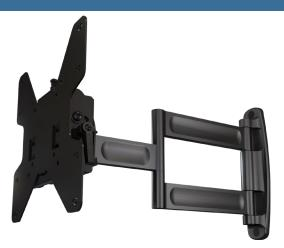
Articulating mount for 13" to 40" displays. Multiple joint arm holds display 2.9" from wall when retracted and 15.4" when fully extended. Smooth tilt adjustments of +15° (forward) and -5° (back) and 2.5° side-to-side roll facilitates a variety of viewing angles and perfect positioning. Makes a secure installation quick and easy, simply hang the screen and turn the pre-assembled securing screw to lock in place. Integrated cable management for clean look.
