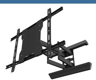
Articulating mount for 37" to 70" flat panel displays. Multiple joint arms hold display 2.5" from wall when retracted and 15.5" when fully extended. Smooth tilt adjustments of +15° (forward) and -5° (back) with a locking knob and 3° side-to-side roll facilitates a variety of viewing angles and perfect display positioning. Makes a secure installation quick and easy, simply hang the display and turn the pre-assembled securing screws to lock in place. Integrated cable management for clean look.
