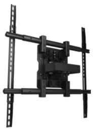
Ceiling mount box and universal screen adapter assembly for 37" to 80" displays. Attaches to standard 1.5" threaded extension columns. Continuous tilt of 15° forward with 360° rotation. Makes a secure screen installation quick and easy, simply hang the display and turn the pre-assembled securing screw to lock the universal adapter in place. Compatible with all 1.5" NPT threaded pipe.
