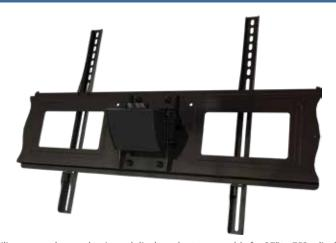
Ceiling mount box and universal display adapter assembly for 37" to 75"+ displays. Attaches to standard 1.5" threaded extension columns. Continuous tilt of 20° forward with 360° rotation. Pin-locking pre-set tilt positions at 5°, 10°, 15° and 20°. Makes a secure display installation quick and easy, simply hang the display and turn the pre-assembled securing screw to lock the universal adapter in place. Compatible with all 1.5" NPT threaded pipe.
