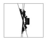
1111 15° forward and 5° back tilt for optimal viewing angles.
