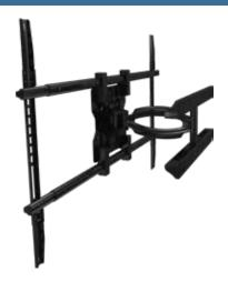
Pivoting mount for 37" to 80"+ flat panel displays. Swinging arm holds display 3.5" from wall and extends up to 14.5". Smooth tilt adjustments of 15° forward and 5° back with a locking knob for a variety of viewing angles. 3° side to side roll for perfect positioning. Makes a secure installation quick and easy, simply hang the display and turn the pre-assembled securing screw to lock in place. Integrated cable management for clean look.
