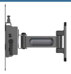
Pivoting mount for 13" to 49" flat panel displays. Swinging arm holds display 2.8" from wall and extends up to 7.9". Smooth tilt adjustments of 15° forward and 5° back with a locking knob for a variety of viewing angles. 5° side to side roll for perfect display positioning. Makes a secure installation quick and easy, simply hang the display and turn the pre-assembled securing screw to lock in place. Integrated cable management for clean look.
