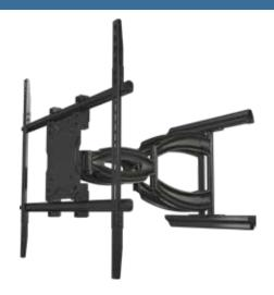
Articulating mount for 37" to 80" displays. Multiple joint arms hold displays  $3.4^{\prime\prime}$  from wall when retracted and 27" when fully extended. Smooth tilt adjustments of +15° (forward) and -5° (back) with a locking knob and 3° side-to-side roll facilitates a variety of viewing angles and perfect positioning. Makes a secure installation quick and easy, simply hang the display and turn the pre-assembled securing screws to lock in place. Integrated cable management for clean look.
