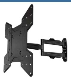
Articulating mount for 13" to 55" display. Multiple joint arm holds display 2.7" from wall when retracted and 21" when fully extended. Smooth tilt adjustments of +15° (forward) and -5° (back) with a locking knob and 3° side-to-side roll facilitates a variety of viewing angles and perfect positioning. Three attachment points for wood studs and four attachment points for concrete walls provide additional security. Integrated cable management for clean look.
