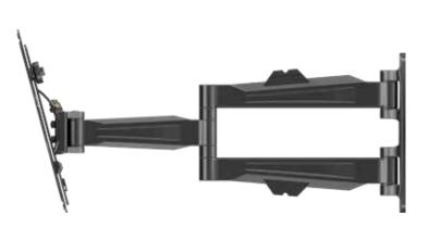
Articulating mount for 13" to 49" displays. Multiple joint arm holds display 2.5" from wall when retracted and 21" when fully extended. Smooth tilt adjustments of +15° (forward) and -5° (back) with a locking knob and 3° side-to-side roll facilitates a variety of viewing angles and perfect positioning. Three attachment points for wood studs and four attachment points for concrete walls provide additional security. Integrated cable management for clean look.
